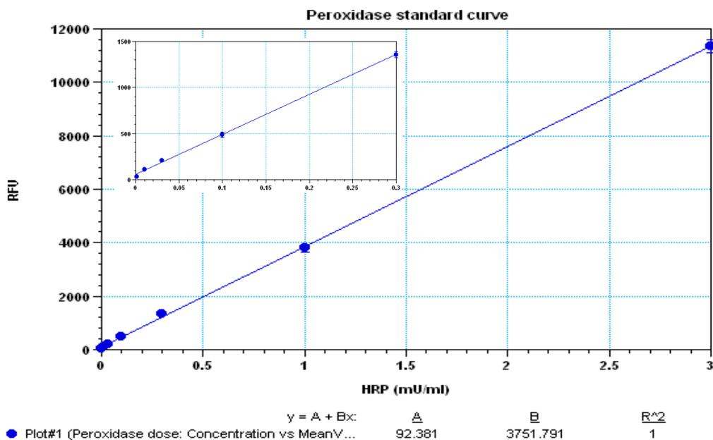
**Figure 1.** HRP dose response was measured with the Amplitude™ Fluorimetric Peroxidase Assay Kit in a 384-well black plate using a Gemini fluorescence microplate reader (Molecular Devices). As low as 10  $\mu\text{U}/\text{mL}$  of peroxidase can be detected with 30 minutes incubation time (n=3). The insert shows the low levels of HRP detection.
